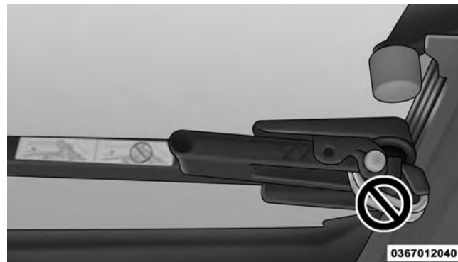
Improper Clamp Position
