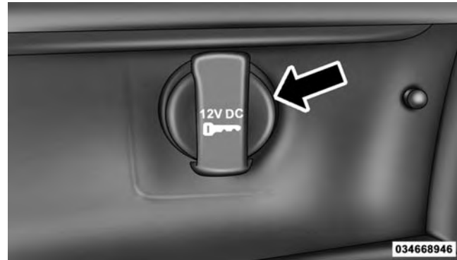
Front Power Outlet
