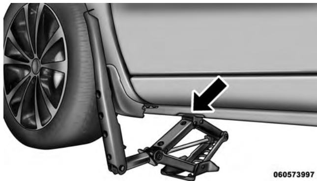
Jack Engaged (Front Jacking Location)
