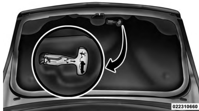
Trunk Internal Emergency Release
