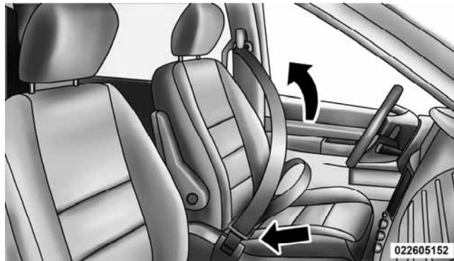
Removing Slack from Belt
