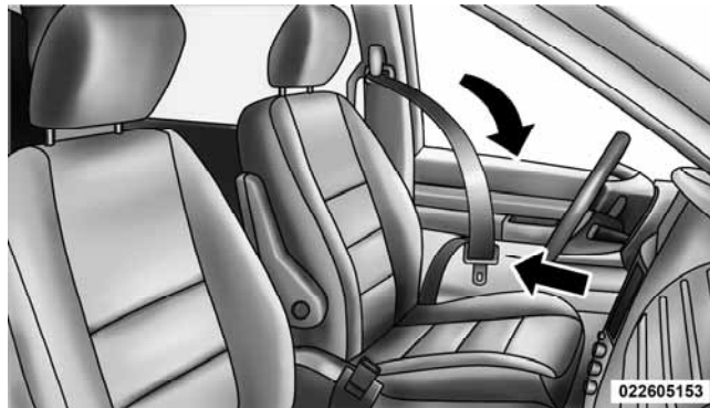
Pulling Out Belt and Latch Plate
