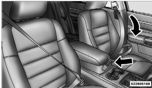
Inserting Latch Plate into Buckle
