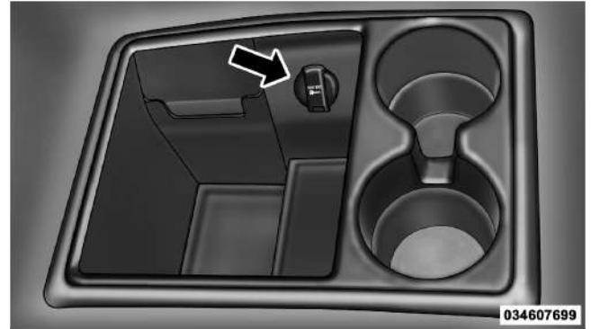
Power Outlet — Floor Storage Bin
